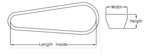
$\begin{array}{ll} \text{Datum Llength} = 780 \\ \text{Height} &= 8 \\ \text{Length inside} &= 750 \\ \text{Width} &= 13 \end{array}$
